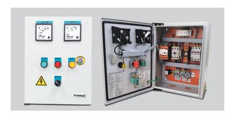
D - Type of control panels are designed to support starting of 3 phase-3 wire Oil Filled / Water Filled / Resin filled submersible motors / Electrical Induction motors. It's an Auto / manual operation design with MCB incomer, ON / OFF Push buttons, power contactor, Electronic pump protection relay, ON delay timer, Surge protectors, trip indication and panel monitoring indications in a sheet steel enclosure with lock & key.
