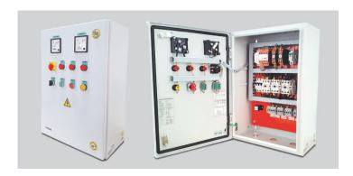
P - Type of control panels are designed to support starting of 3 phase-6 wire submersible / Electrical Induction motors. It's an Auto / manual operation design with MCB/ MCCB incomer, ON / OFF Push buttons, power contactors, Electronic pump protection relay, ON delay timer, Surge protectors, phase-phase voltage and current monitoring provision, trip indication and panel monitoring indications in a sheet steel enclosure with lock & key.
