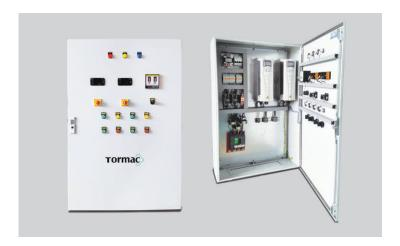
This type of control panels are designed to support starting 3 phase -3 wire submersible / Electrical Induction motors with a smooth starting curve with reduced starting currents & Voltages. It works on the principle of varying the frequency and voltage supplied to the electric motor.
