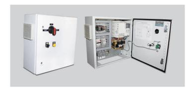
This type of control panels are designed to operate motors with energy drawn from photovoltaic cells (PV). The inverter is customized to operate in dual supply mode, so the grid connected supply is used in the absence of energy from PV cells. A four-pole changeover switch enables switching between the two supply modes.
