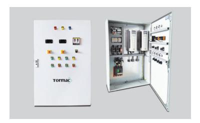
This type of control panels are designed to support starting 3 phase - 3 wire submersible / Electrical Induction motors with a smooth starting curve with reduced starting currents & Voltages.
