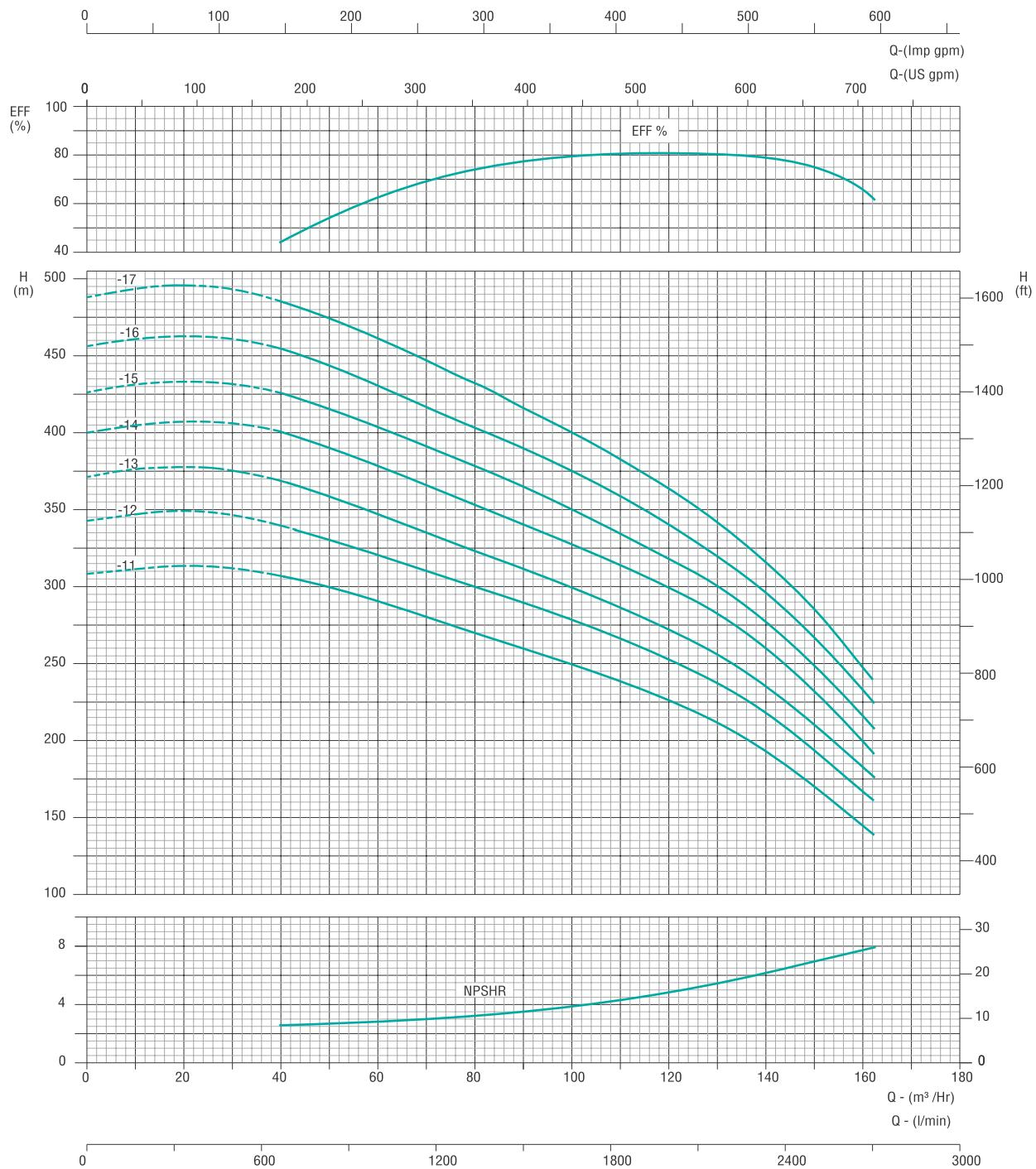
Curve tolerance according to ISO 9906:2012, Grade 3B
