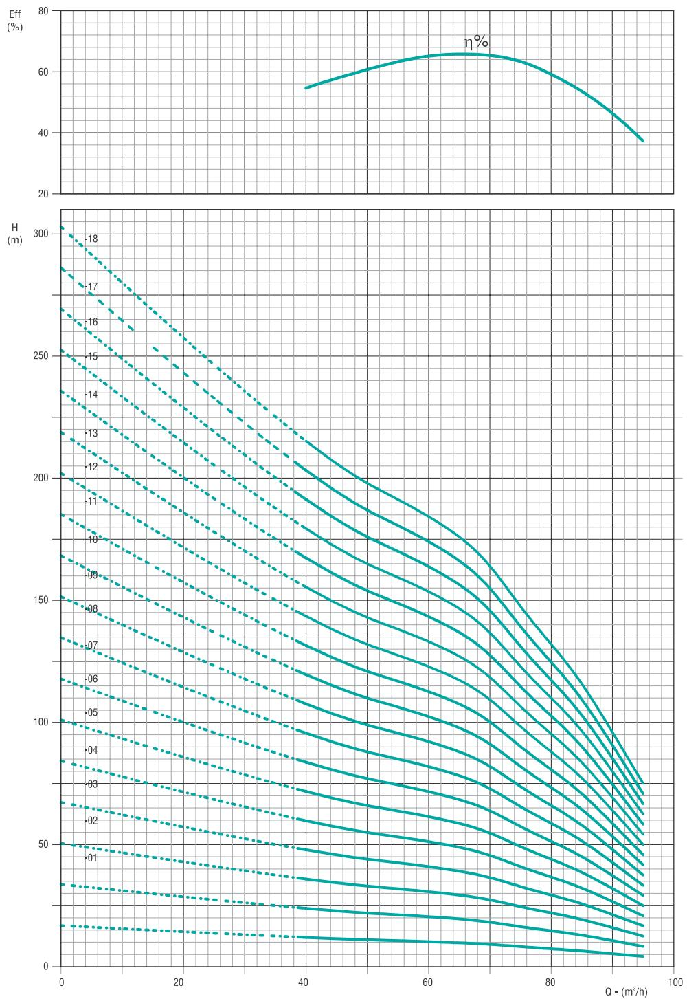
Curve tolerance according to ISO 9906:2012, Grade 3B
