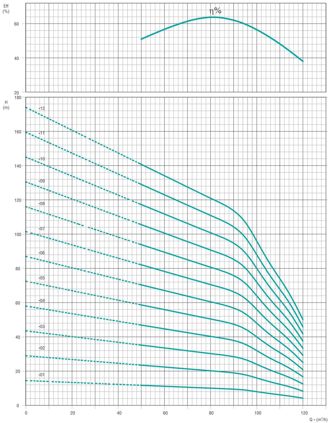
Curve tolerance according to ISO 9906:2012, Grade 3B
