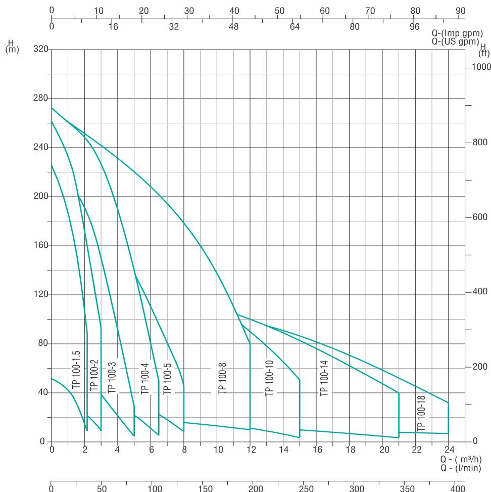
Curve tolerance according to ISO 9906:2012, Grade 3B
