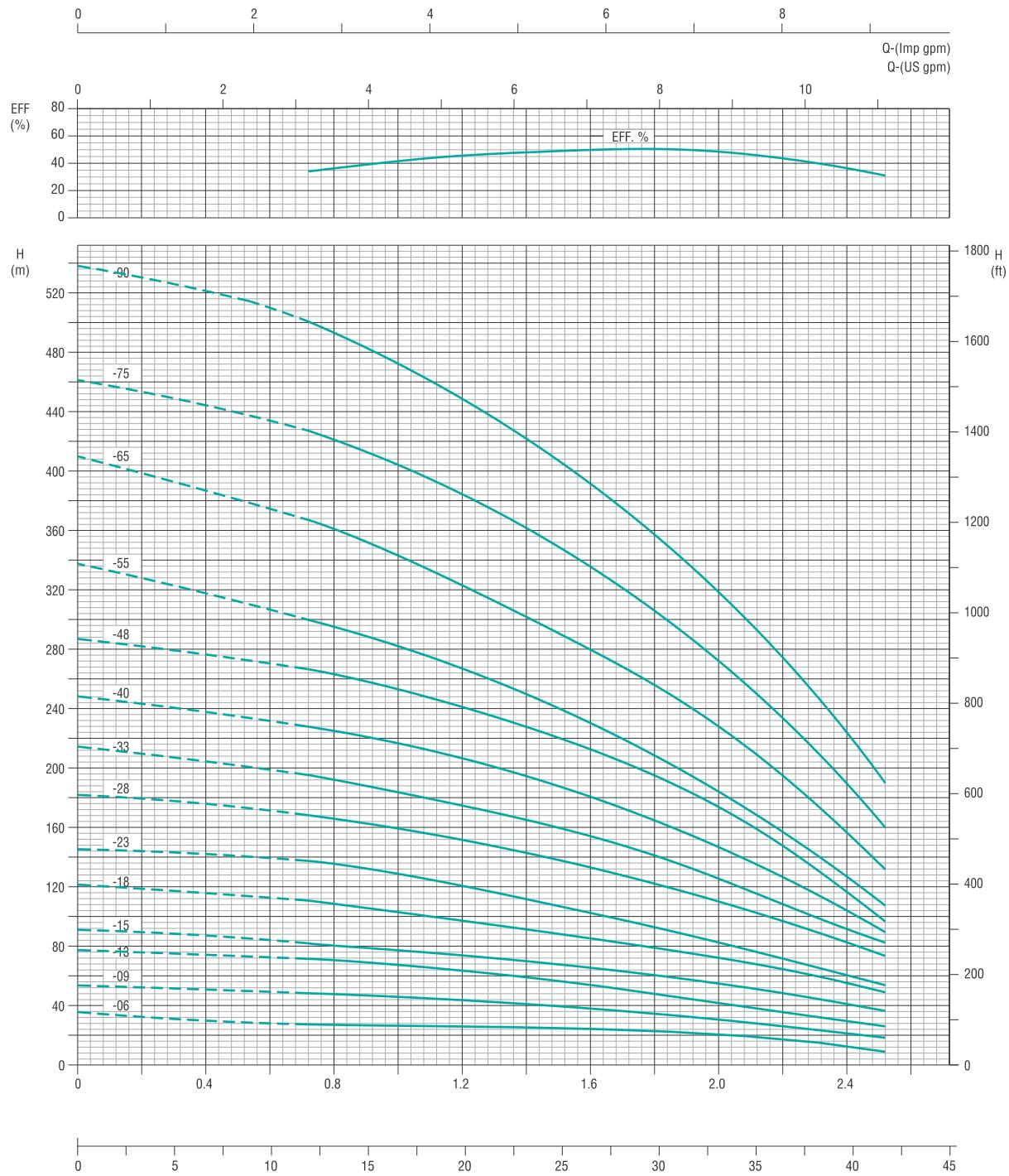
Curve tolerance according to ISO 9906:2012, Grade 3B
