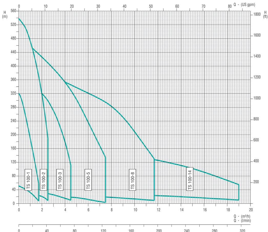
Curve tolerance according to ISO 9906:2012, Grade 3B
