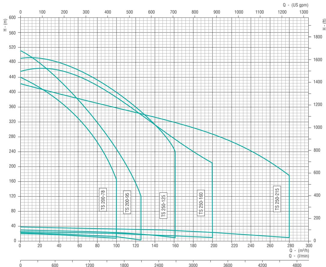
Curve tolerance according to ISO 9906:2012, Grade 3B
