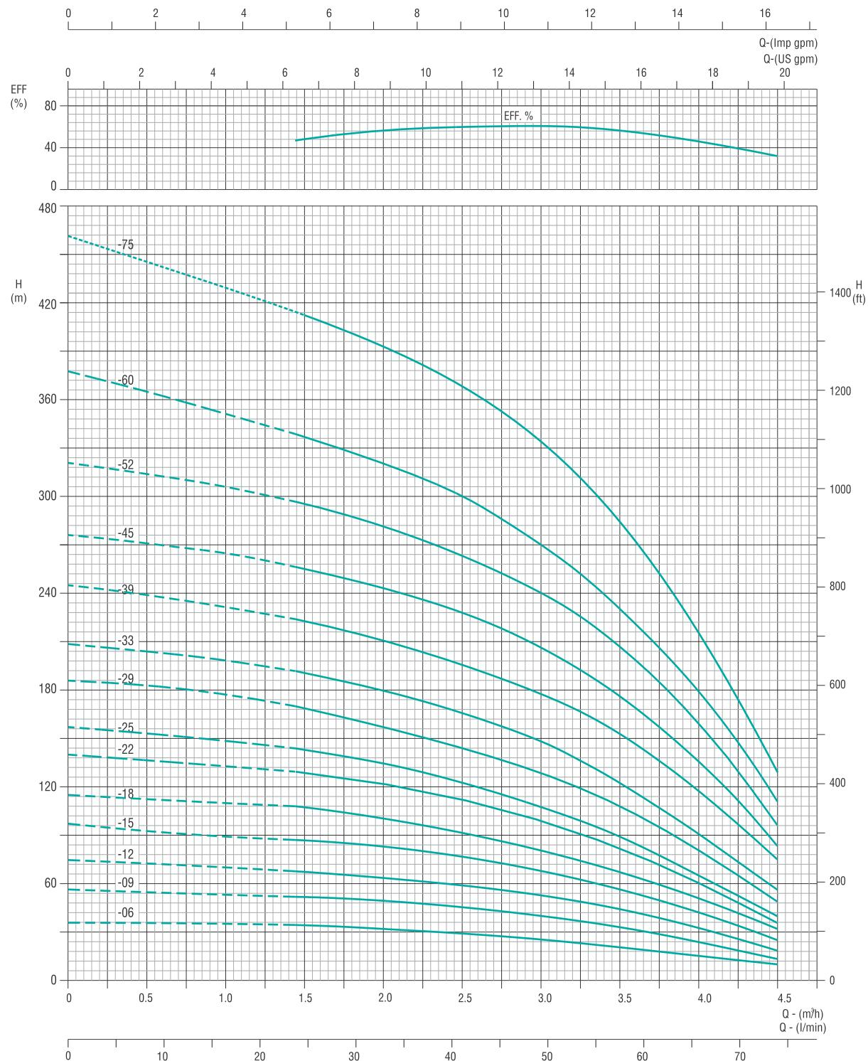
Curve tolerance according to ISO 9906:2012, Grade 3B
